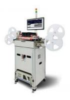
VR20i Post Seal Vision Handler covers multiple vision systems in one machine such as tape seal inspection, mark inspection, package inspection, lead inspection and bottom carrier inspection tape. Another excellent feature is its fast changeover with quick and easy tape loading for different packages. This unique capability of the multiple vision stations maximizes the production throughput and inspection options for the semiconductor and LED industry
