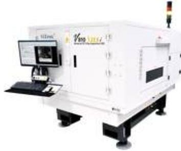
**V810 S2EXi** can handle boards up to 19 x 24", an increase of 10 percent over its predecessor – the V810 S2 system. It supports boards up to 280mils thick and 4.5kgs. With the introduction of the Motorized X-ray Tube and Motorized Filter Height Sensor (FHS), V810 S2EXi offers greater top clearance up to 50mm and bottom clearance up to 70mm. High accuracy and repeatability are achieved with this motorized closed-loop design.
